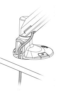
To replace the cover, first align the markings on the cover and arm and then slide to lock into place.
